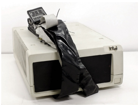
Figure 1. Intel I2ICE, one of the first in-system debuggers for Intel 80386 processors (recycledgoods.com/intel-series-iv-emul-system-iii514b.html)
